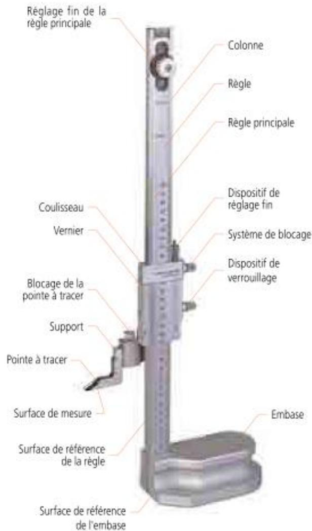
Fig I.6 – Trusquin a vernier.
